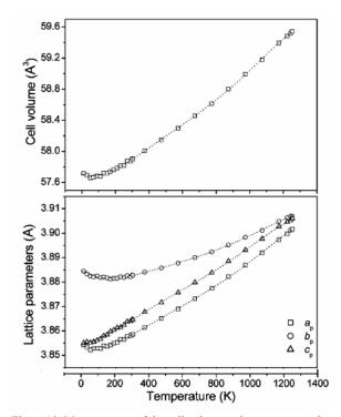
Figure 10: Measurements of the cell volume and parameters as they vary with temperature for PrGaO<sub>3</sub>. (The measurements and graphs are taken from Vasylechko *et al.* 2005). The NTE window between *circa* 12K and 50K is evident.
