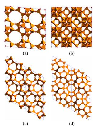
Figure 3: The polyhedral structures of (a) CHA and (b) FAU, (c) ERI and (d) MWW. In all cases the visualisation is in 2X2 cell format showing the (001) plane.
