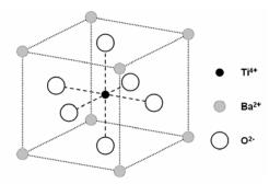
Figure 4: The idealised 'crystal perovskite structure' of BaTiO<sub>3</sub>. The TiO<sub>6</sub> tetrahedral units (i.e. the units with the O at the vertices and the Ti at the centre) illustrated in this figure are distorted at room temperature and become more regular as the temperature is increased, a process which results in a reduction in volume (i.e. NTE).
