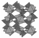
Figure 2: The structure of an  $AM_2O_7$  member. The large light gray polyhedra represent  $M_2O_7$  units while the smaller dark gray polyhedra represent  $AO_6$  units.
