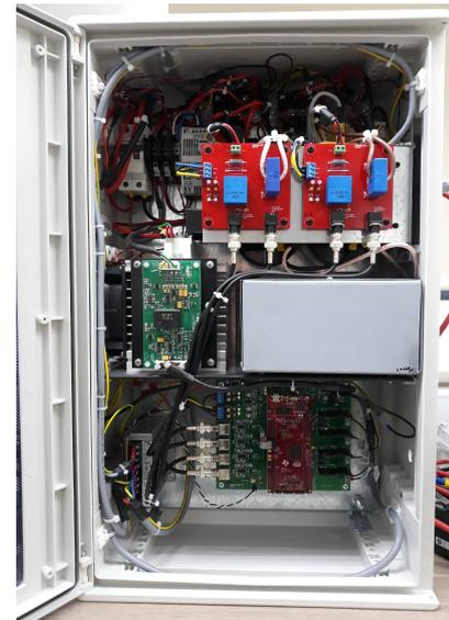
Figure 2: A microgrid DC-to-DC converter implemented for the DC microgrid in the IEPC labs.
